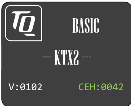
Figure 4: Start screen of a device that supports "BASIC" functionality (Mode A/C/S only)
