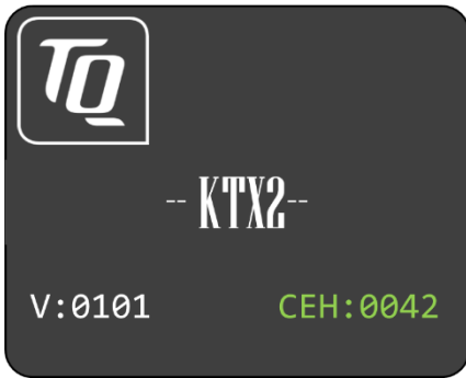
Figure 3: Start screen of a device with enabled "Extended Squitter ADS-B out" feature
