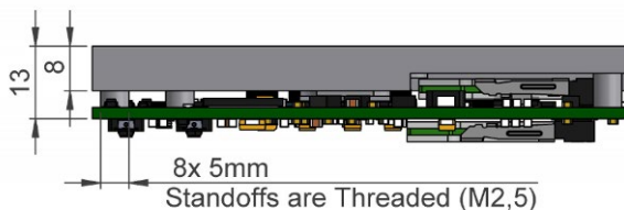
Illustration 7: TQMx80UC-HSP Heat Spreader
