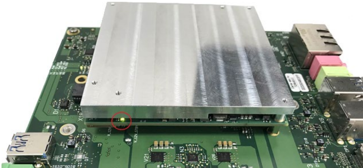
Illustration 16: TQMx80UC green Debug LED
