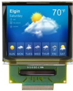
Figure 33: OLED display NHD-1.69-160128G
