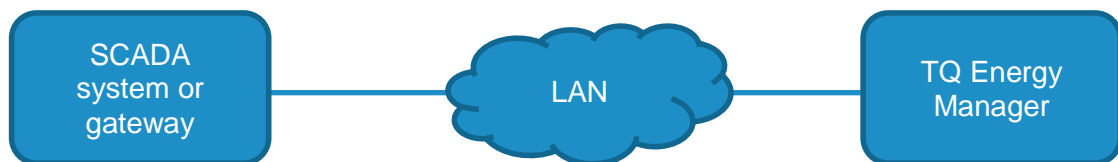
Figure 2 - Block diagram for Ethernet usage
