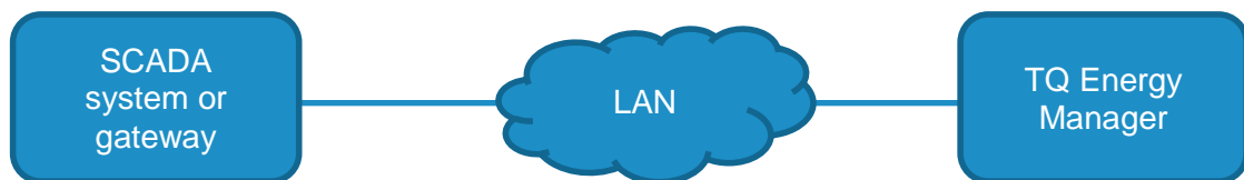
Figure 2 - Block diagram for Ethernet usage
