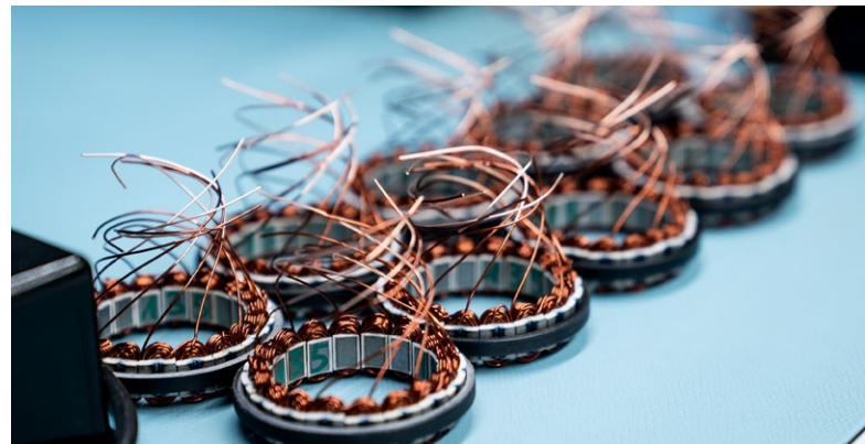
Production of frameless motors from TQ-RoboDrive in Inning am Ammersee
