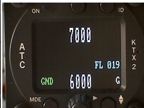
GND-switch installed, on GND
