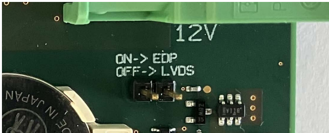
Illustration 7: Config jumper: eDP or LVDS
