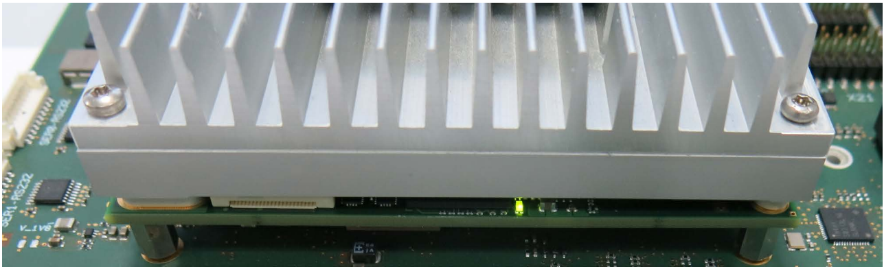
Figure 16: TQMx120 Debug LED
