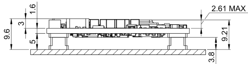
Figure 18: TQMLS1028A dimensions, side view
