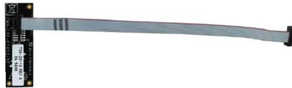
Figure 39: NXP Code Warrior TAP adapter (source NXP)
