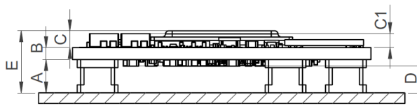
Figure 34: TQMa8Xx dimensions, side view
