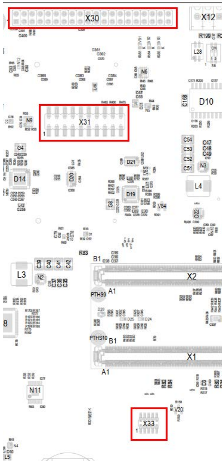
Figure 38: Position of headers X30, X31, X33
