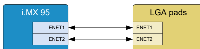
Figure 8: Block diagram 1G Ethernet (RGMII)
