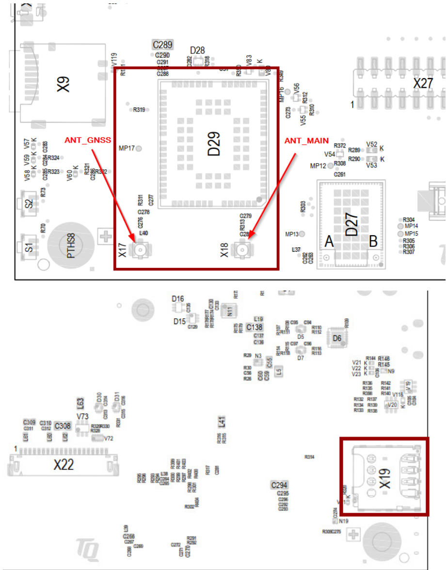
Figure 29: Position IoT radio module + u.FL + Micro-SIM card port
