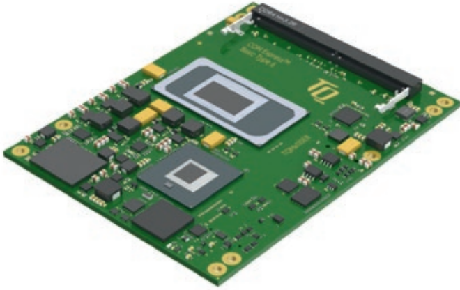
COM Express® Basic Type 6 Module with 11 th Generation Intel® Core™ Processors.
