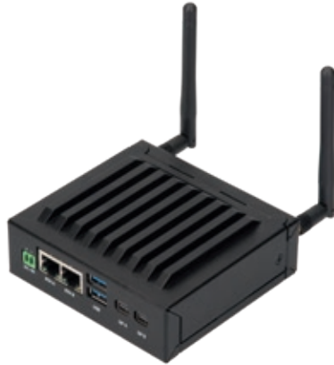
Ultra compact BoxPC platform for embedded PC applications and IoT edge gateways.
