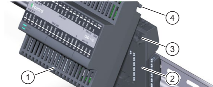
Fig. 6: Install the electronic module
