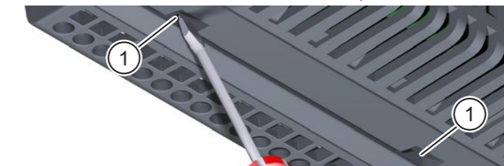
Fig. 9: Uninstalling the electronic module
