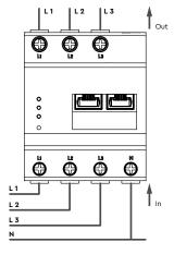
The device operates on phase L1
