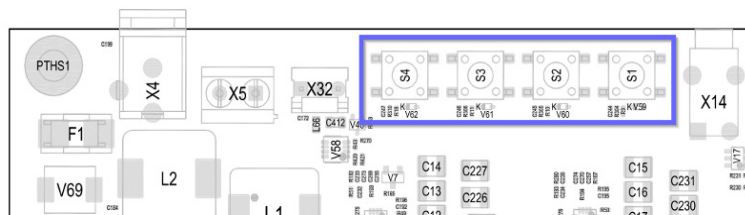
Figure 46: Position of GP buttons, S1, S2, S3 and Reset button, S4
