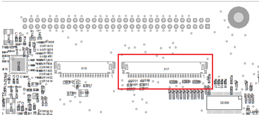
Illustration 26: Position of LVDS, X17
